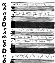
FIG. 9.—Section of coal strata. a , bind; b , shale; c , rock; D , coal; e , seat, or fire-clay.
